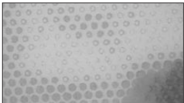
Photo 8 – These tones show the doughnut center typical of gravure printing. This sample used laser engraved cylinders.
