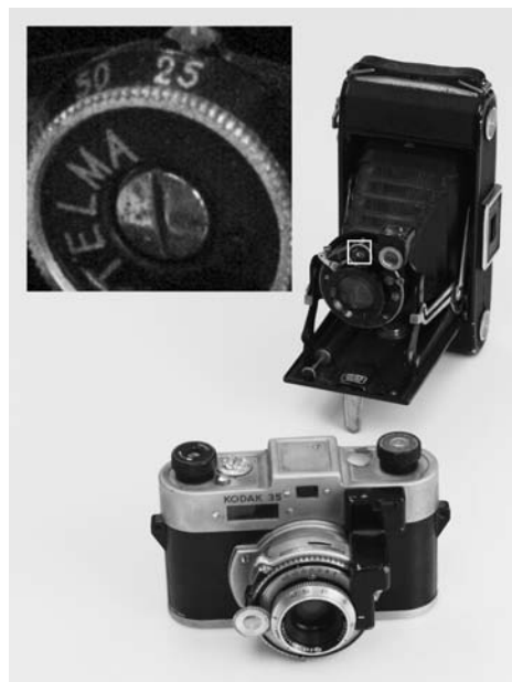
Figure 4. The enlarged image detail (top left) corresponds to the small area marked by the white square in the larger original photo of the two cameras. This is a 150x150 pixel portion of the larger 3700x5000 scan made with the Betterlight 4000E back.
