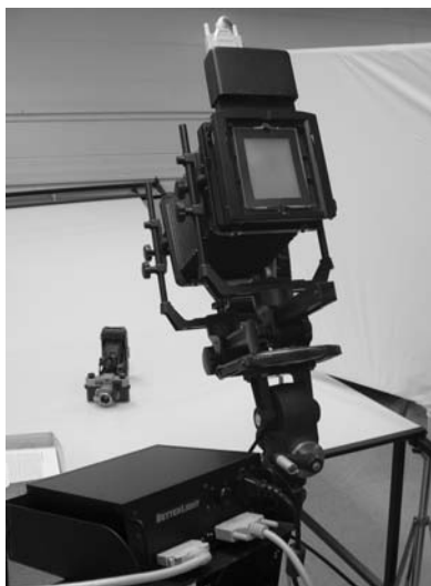
Figure 3. The Betterlight system includes a scanning sensor that is inserted into the film back compartment of a 4x5 inch view camera. This sensor (top) is connected with a cord to a control box (bottom left). This control box is connected to a Macintosh or PC computer running the "Viewfinder" scanning software.
