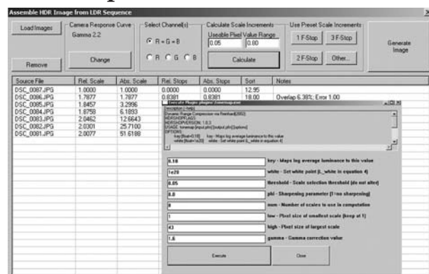
Figure 7- Assemble HDR Image from LDR Sequence and the Reinhard tone map filter windows in HDR Shop
