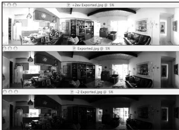
Figure 11- Bracketed panoramic images ready to be converted to a HDR file in Photomatrix
